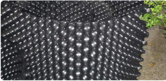
Yuan Da **Dimpled Wall Drains** are made from a cusped core, bonded to a high quality nonwoven geotextile. The core's high compressive strength resists high loads from in-fill and formwork. Its stud-shaped dimples provide an air chamber between the sheet and wall to rapidly channel water from grade to the footer drainage system. It is resistant to saline solutions, alkalis and acids.
